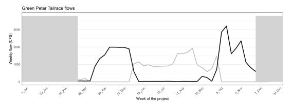
Figure E-4. Green Peter Dam Tailrace powerhouse outflow (gray line) and spill outflow (black line) for 2023.
