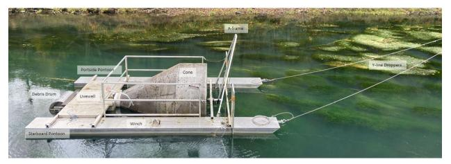
Figure H-1. Labeled image of a rotary screw trap showing parts and terminology.
