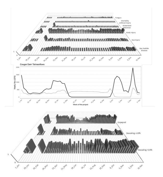
Figure 25. Proportion of captured juvenile Chinook salmon displaying injuries by type (top panel), operations data from Cougar Dam showing cfs of spill (black line) and Powerhouse flow (gray line) outflows (middle panel), and proportion of captured juvenile Chinook salmon displaying descaling and copepod injuries (bottom panel) from January 1, 2023, through November 30, 2023.
