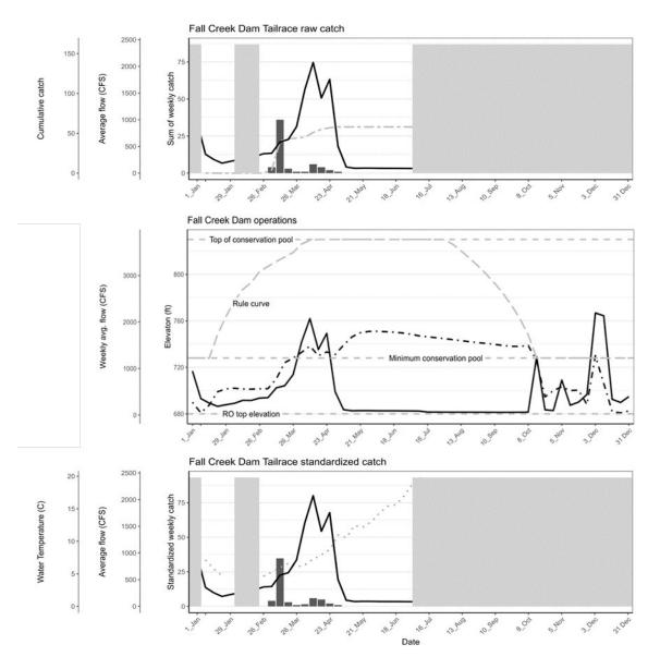
Figure 30. Raw catch (top panel), Fall Creek Dam forebay and intake elevations (middle panel), and weekly standardized catch (bottom panel) of natural origin juvenile Chinook salmon at the Fall Creek Dam Tailrace site with RO outflow (black line), forebay elevation (black dot dash line), intake elevations (gray dash line), cumulative catch (gray dot dash line), stream temperature (gray dot line), and non-sampling weeks shaded out (gray) for January 1, 2023, through July 15, 2023.
