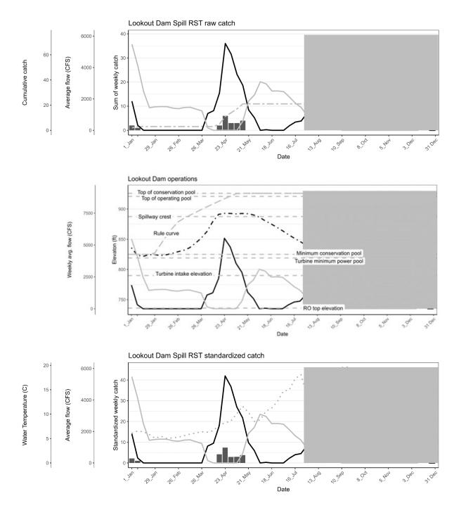
Figure 41. Raw catch (top panel), Lookout Point Dam forebay and intake elevations (middle panel), and weekly standardized catch (bottom panel) of natural origin juvenile Chinook salmon at Lookout Dam Tailrace Spill trap with spill (black line), Powerhouse outflow (gray line), forebay elevation (black dot dash line), intake elevations (gray dash line), stream temperature (gray dots), and cumulative catch (gray dot dash line) from January 1, 2023, through July 31, 2023.
