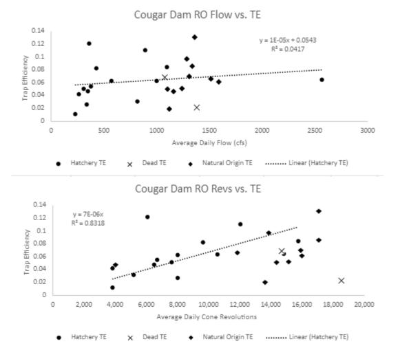
Figure E-13. Cougar Dam Tailrace RO trap efficiency trials versus flows (top panel) and compared to cone flux (bottom panel). Linear regression fit is only to hatchery TE trials in both panels, which is non-significant for flow and significant for cone flux.
