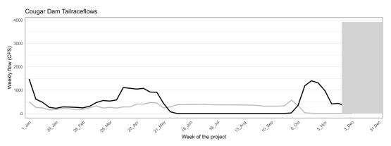
Figure E-11. Cougar Dam Tailrace powerhouse outflow (gray line) and spill outflow (black line) for 2023.
