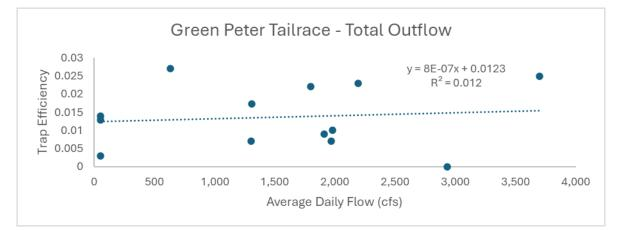
Figure E-5. Green Peter Dam Tailrace trap efficiency trial plots. Linear regression fit is nonsignificant. Plot displays trapping efficiencies versus total outflow.
