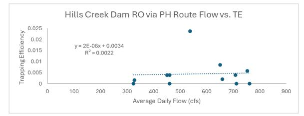
Figure E-27. Hills Creek RO trapping efficiency versus Powerhouse flows.
