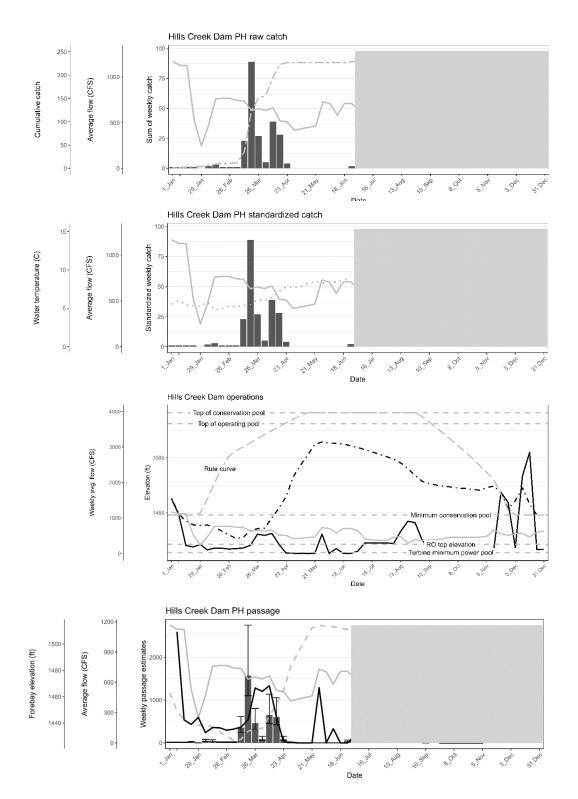
Figure 49. Raw catch (top panel), weekly standardized catch (second panel), Hills Creek Dam operations and features of interest (third panel), and weekly passage estimates (bottom panel) overlayed with Powerhouse outflow (gray line), RO outflow (black line), cumulative catch (gray dash dot line), forebay elevation (black dot dash line) and stream temperature (gray dots) for the PH trap below Hills Creek Dam for sampling from January 1, 2023, through June 30, 2023.
