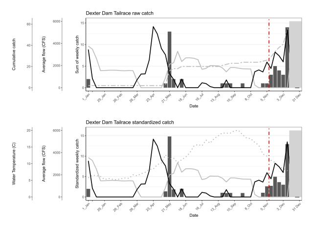
Figure 34. Raw catch Dexter Dam (top panel) and weekly standardized catch (bottom panel) of natural origin juvenile Chinook salmon at the Dexter Dam Tailrace site with spill (black line), Powerhouse outflow (gray line), cumulative catch (gray dot dash line), forebay elevations (black dot dash line), and water temperature (gray dots) January 1, 2023, through December 15, 2023. The red dot dash line denotes when the trap was moved downstream to the new sampling location due to construction.
