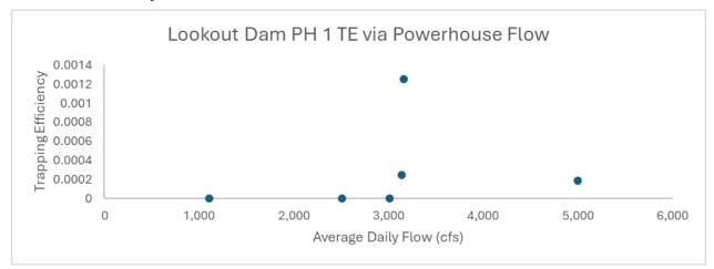
Figure E-21. Lookout Dam Tailrace PH1 trapping efficiency versus the powerhouse flows.
