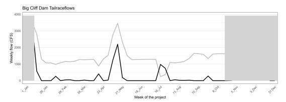
Figure E-1. Big Cliff Dam Tailrace powerhouse outflow (gray line) and spill outflow (black line) for 2023.
