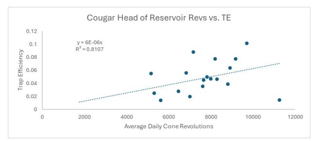
Figure E-15. Cougar Head of Reservoir trap efficiency versus cone flux the day after trial fish were released.
