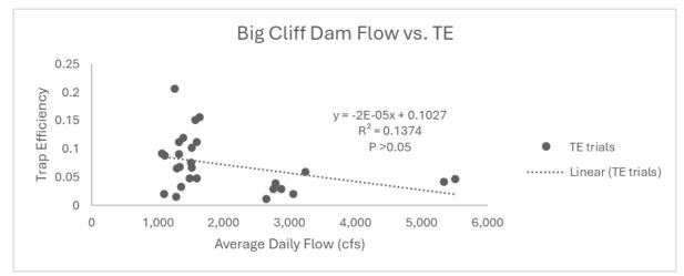
Figure E-2. Big Cliff Dam Tailrace trap efficiency trial plots. Linear regression fit is non-significant. Plot displays trapping efficiencies versus flow levels.
