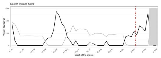
Figure E-17. Dexter Dam Tailrace powerhouse flow (gray line) and spill flow (black line) for 2023. The red dashed line denotes when the RST was moved downstream due to construction.
