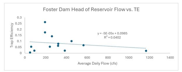
Figure E-9. Foster Dam Head of Reservoir trap efficiency trial plots. Linear regression fit is nonsignificant. Plot displays trapping efficiencies versus flows.
