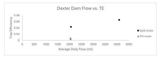
Figure E-18. Dexter Dam Tailrace trap efficiency trial plots versus flow levels for the RST position near the powerhouse (top panel) and downstream near the boat launch (bottom panel).
