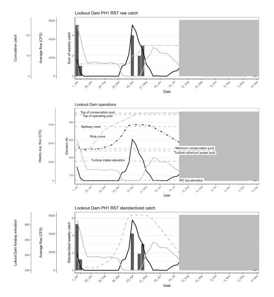
Figure 39. Raw catch (top panel), Lookout Point Dam forebay and intake elevations (middle panel), and weekly standardized catch (bottom panel) of natural origin juvenile Chinook salmon at Lookout Point Dam Tailrace PH1 trap with spill (black line), Powerhouse outflow (gray line), forebay elevation (black dot dash line), intake elevations (gray dash line cumulative catch (gray dot dash line) from January 1, 2023, through July 31, 2023.
