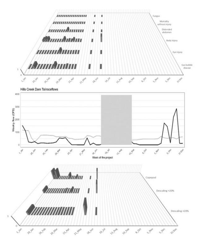
Figure 51. Proportion of captured juvenile Chinook salmon displaying injuries by type (top panel), operations data from the Hills Creek Dam showing cfs of spill (black line) and Powerhouse flow (gray line) outflows (middle panel), and proportion of captured juvenile Chinook salmon displaying descaling injuries and copepods (bottom panel) from January 1, 2023, through June 30, 2023.
