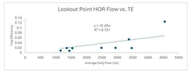
Figure E-24. Lookout Point Head of Reservoir trapping efficiency versus flows.
