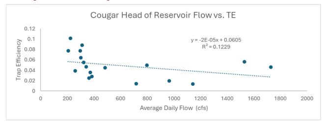
Figure E-14. Cougar Head of Reservoir trap efficiency trials versus flows.
