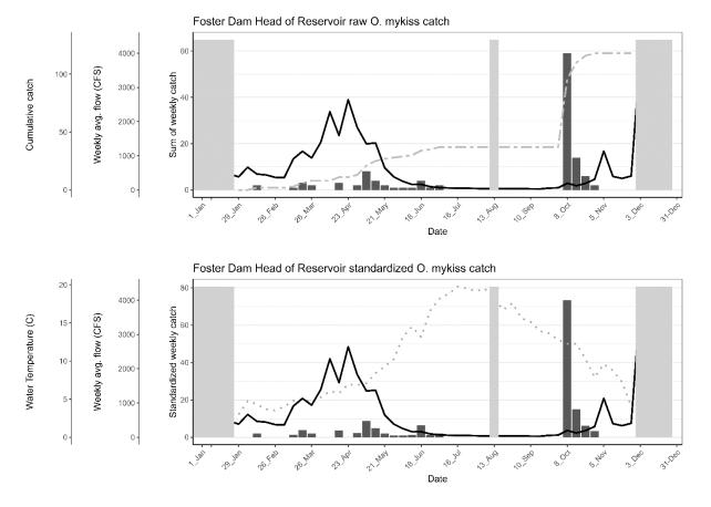
Figure 17. Shows raw (top panel) and weekly standardized (bottom panel) catch of juvenile *O. mykiss* overlayed with stream flow (black line), cumulative catch (gray two dash line), stream temperature (gray dots), and non-sampling weeks shaded out (gray) for January 1, 2023, November 30, 2023.
