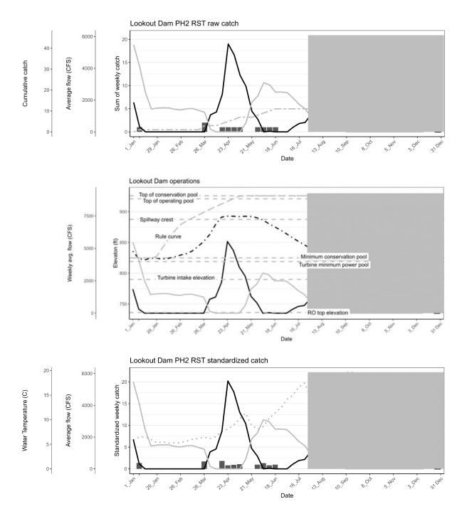
Figure 40. Raw catch (top panel), Lookout Point Dam forebay and intake elevations (middle panel), and weekly standardized catch (bottom panel) of natural origin juvenile Chinook salmon at Lookout Dam Tailrace PH2 trap with spill (black line), Powerhouse outflow (gray line), forebay elevation (black dot dash line), intake elevations (gray dash line), stream temperature (gray dots), and cumulative catch (gray dot dash line) from January 1, 2023, through July 31, 2023.
