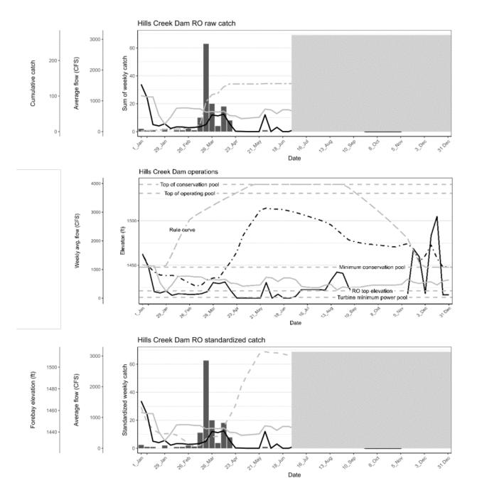
Figure 48. Raw catch (top panel) and weekly standardized catch (bottom panel) overlayed with RO outflow (black line), Powerhouse outflow (gray line), cumulative catch (gray dash dot line), and forebay elevation (gray dash line) for the RO trap below Hills Creek Dam for sampling from January 1, 2023, through June 30, 2023. The middle panel shows Hills Creek Dam operations and features of interest with RO outflow (black line), Powerhouse outflow (gray line), and forebay elevation (black line).
