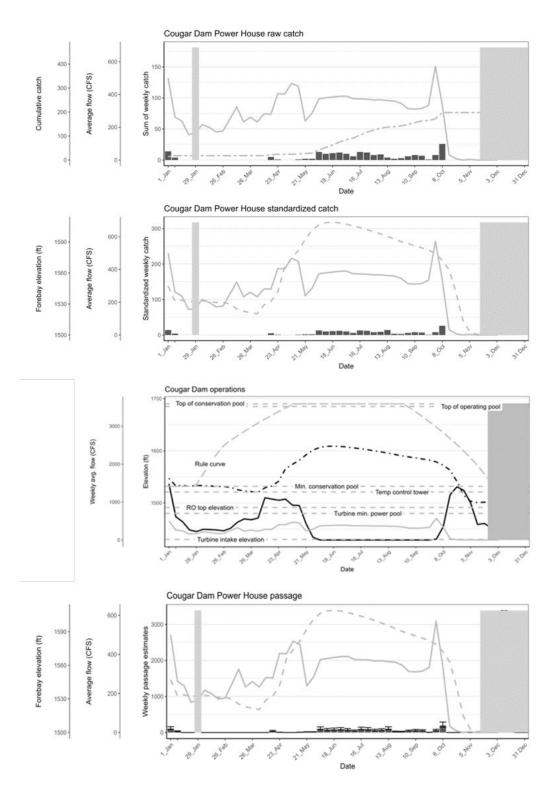
Figure 22. Raw catch (top panel), weekly standardized catch (second panel), Cougar Dam operations (third panel), and weekly passage estimates (bottom panel) overlayed with Powerhouse outflow (gray line), cumulative catch (gray dash dot line), forebay elevation (black dot dash line), water temperature (gray dot line), and non-sampling weeks shaded out (gray) and non-sampling weeks shaded out (gray) for the Powerhouse traps at Cougar Dam from January 1, 2023, through November 30, 2023.
