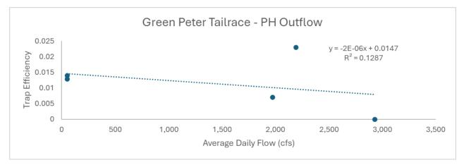
Figure E-7. Green Peter Dam Tailrace trap efficiency trial plots. Linear regression fit is nonsignificant. Plot displays trapping efficiencies versus powerhouse flows.
