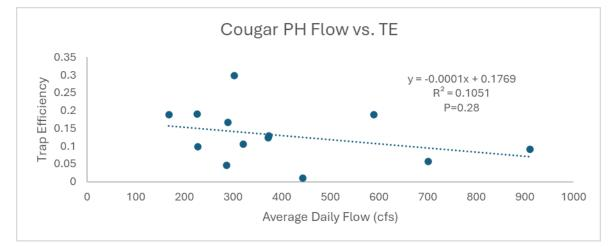
Figure E-12. Cougar Dam trap efficiency trial plots versus flows. Cougar PH linear regression fit is slightly negative with increasing flow.
