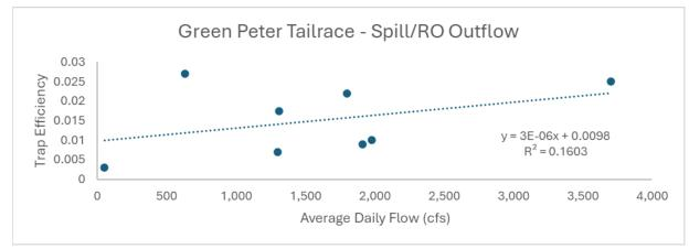
Figure E-6. Green Peter Dam Tailrace trap efficiency trial plots. Linear regression fit is nonsignificant. Plot displays trapping efficiencies versus spill/RO flows.
