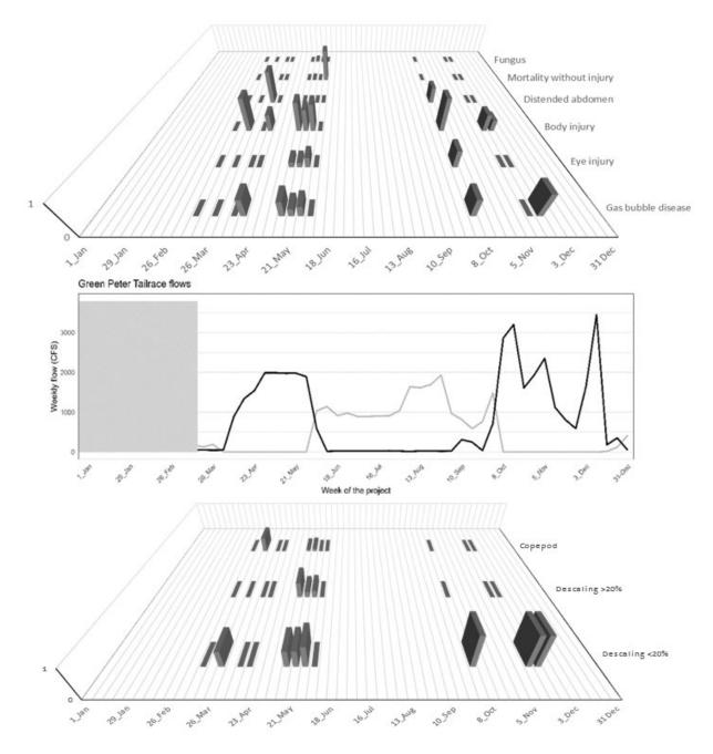
Figure 13. Injury rate of captured Chinook salmon below Green Peter Dam displaying proportion of fish with injuries by type (top panel) and descaling injuries and copepod presence (bottom panel). The middle panel shows spill (black line) and Powerhouse flow (gray line) at Green Peter Dam from 2023.
