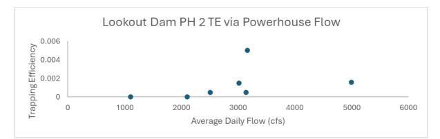
Figure E-23. Lookout Dam Tailrace PH2 trapping efficiency versus powerhouse flows.
