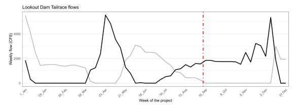
Figure E-20. Lookout Dam Tailrace powerhouse flow (gray line) and spill flow (black line) for 2023. The red dot dashed line denotes when the powerhouse RSTs were moved to a side-by-side orientation for safety.
