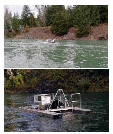
Figure H-14. Hills Creek Dam – Regulating Outlet sampling at high (top) and medium (bottom) flow.
