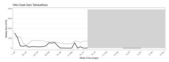
Figure E-26. Hills Creek Dam Powerhouse flow (gray line) and spill flow (black line) for 2023.
