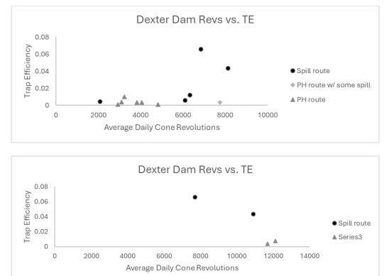
Figure E-19. Dexter Dam Tailrace trap efficiency trial plots versus cone flux for the RST position near the powerhouse (top panel) and downstream near the boat launch (bottom panel).
